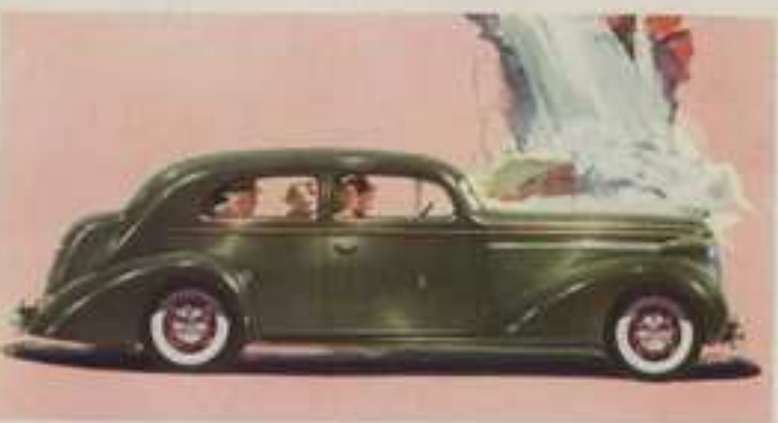
NASH AMBASSADOR SIX VICTORIA SEDAN 121-inch wheelbase Valve-in-head Twin-Ignition 95 Horsepower Motor
