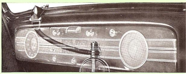
WINDSHIELD DEFROSTER—A new Packard unit. It forces a stream of hot air across the windshield in front of the driver, keeping the glass free of mist, sleet and frost. Independent of the car heater, it can be used at any time. Its use will add immeasurably to the pleasure and safety of driving in bad weather, summer or winter. Installed price \$6.75.
