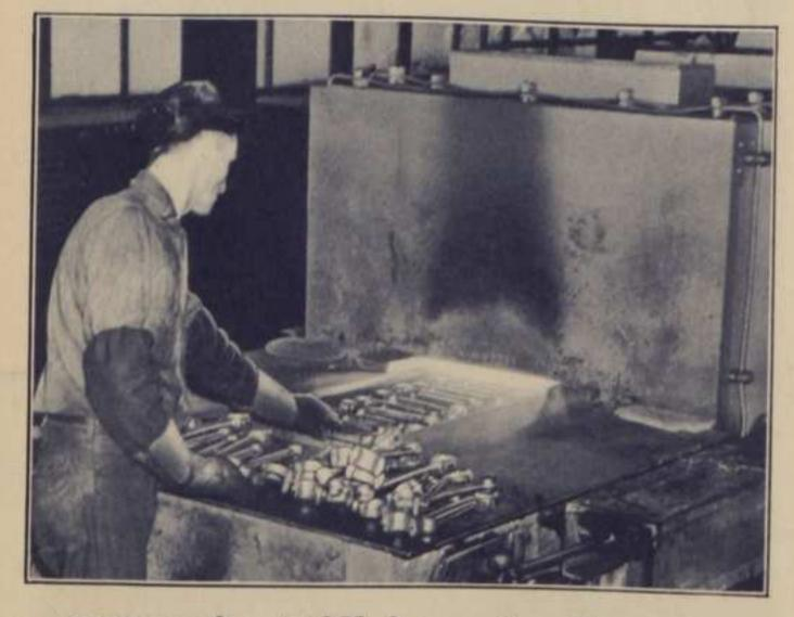
... comes another rigid Nash inspection. Every connecting rod ... every camshaft ... every steering knuckle ... every other Nash forging must meet any one of several tests for hardness.
