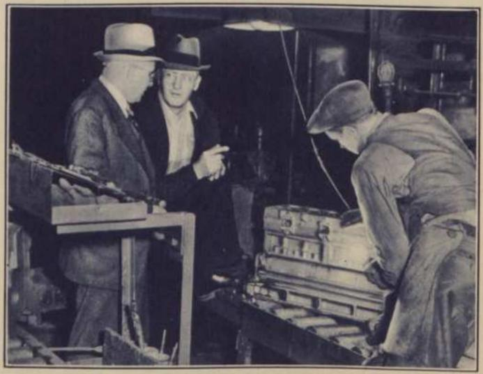
... and step into the Nash forge—where those parts of the engine which are not cast are forged from fine steel. Let's take, for instance, the connecting rod which begins as a bar of very tough high-carbon steel.
