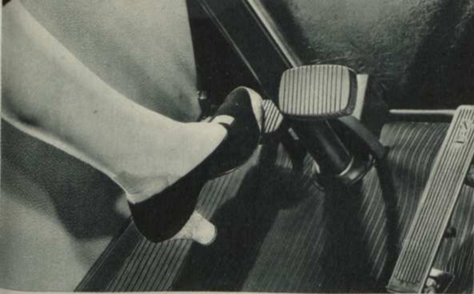
CLUTCH PEDAL STARTER . . . disengages transmission in starting, hence battery never has to turn over gears in cold, stiff grease. The same pedal controls both clutch and starter, under the left foot, so that the driver has both hands free, and the right foot ready to operate foot brake or accelerator if needed. A great convenience when starting and an extra value safety feature!
