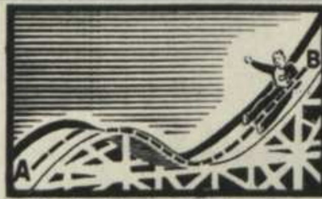
Fuel mixture which has to travel down, then up, as the boy in this illustration, is delayed reaching the cylinders.
