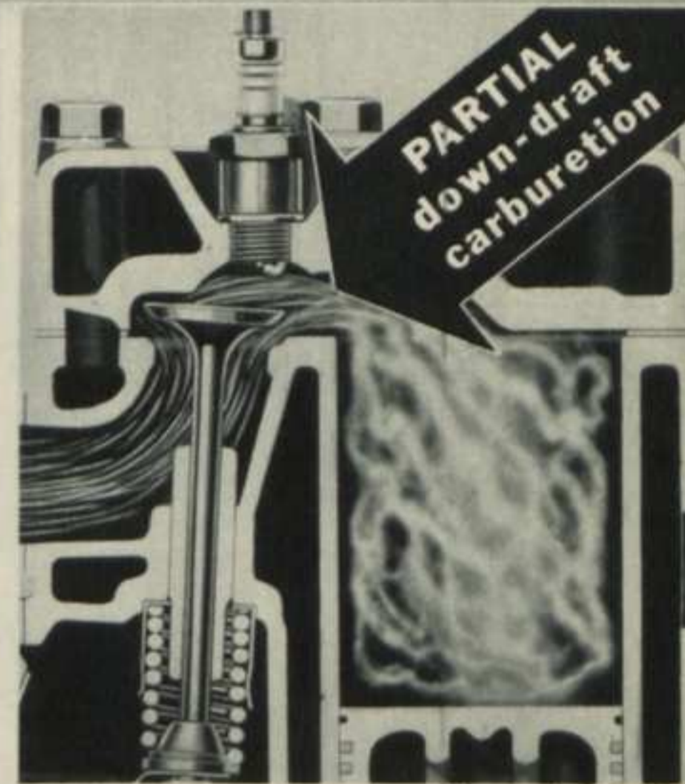
Fuel mixture which has to travel down, then up, as the boy in this illustration, is delayed reaching the cylinders.
