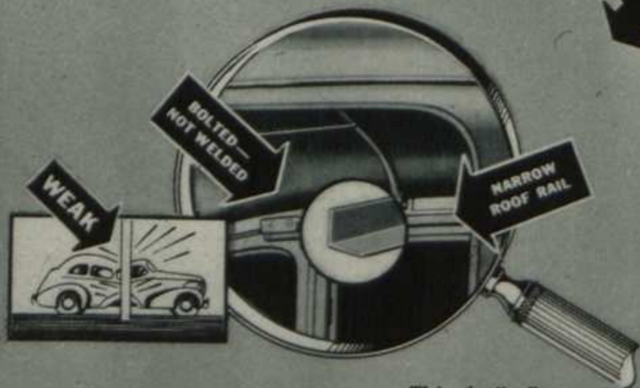
This frail, flange-type roof rail construction used in many competitive "steel bodies" — cannot compare for strength with Nash.
