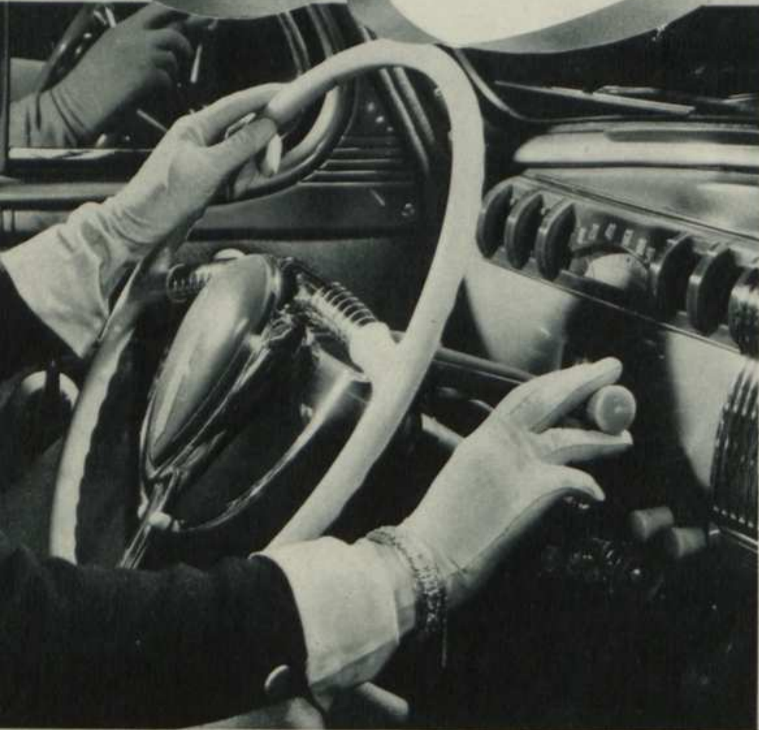
NASH'S STEERING POST SHIFT is standard equipment on all models. New improvements provide smooth, rapid shifting under all conditions. Specially cushioned against metallic noises . . . there's no sticking . . . no clanking . . . no coaxing to find the right gear. All gears in constant mesh to promote smooth, rapid shifting at all times. Silencing bushings are also used in the linkage.
