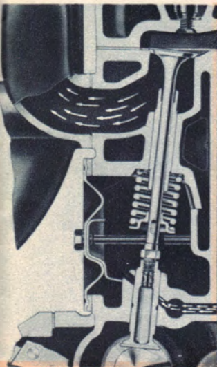
Angle-set valves—for more efficient and complete combustion, improved economy.
