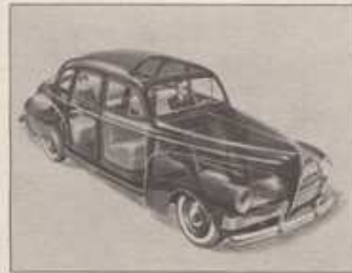
Frame and body are one strong unit, a new type of construction adapted from the latest Streamliner and Streamliner developments. Safer, more rigid, the unit is squeak-proof, twist-proof, rattle-proof. Unusual dead weight has been eliminated, adding to the handling ease and sensational economy.
