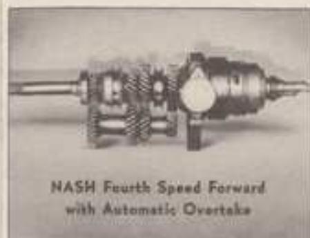
The famous Nash Fourth Speed Forward cuts its automatic 11 to 15 miles per hour to reduce engine speed 50 per cent. Runs up to 21 per cent on gas, up to 10 per cent on oil. The Automatic Overtake comes in when you depress the accelerator to the limit, shifts you ahead in traffic or for emergencies.
