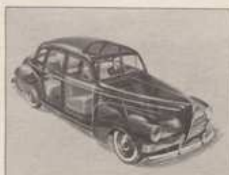
Frame and body are one strong unit, a new type of construction adapted from the latest Streamliner and Standard Development. Safer, more rigid, the unit is squawk-proof, twist-proof, rattle-proof. Unless dead weight has been eliminated, adding to the handling ease and seasonal economy.
