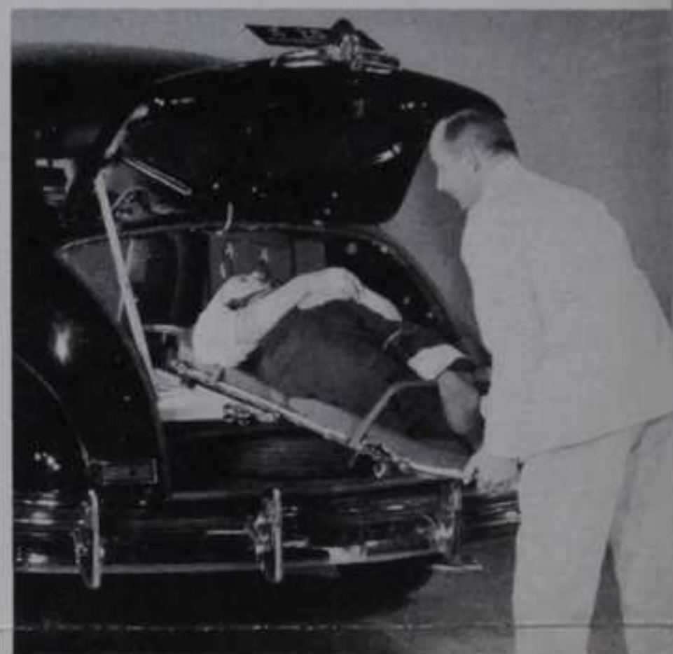
ROLLING STRETCHER INTO CAR. Stretcher is set on tracks, then rolled into place. Winged nut locks stretcher in place, prevents it rolling backwards. Trunk door is lowered and Nash ambulance is ready to proceed.
