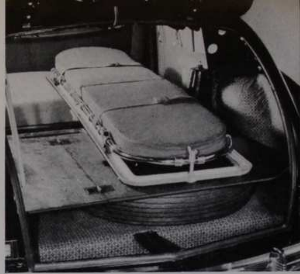
ROLLER STRETCHER in position on stretcher track. Stretcher is anchored into place by means of a bracket and winged nut. Special straps on stretcher hold patient securely while car is in motion.
