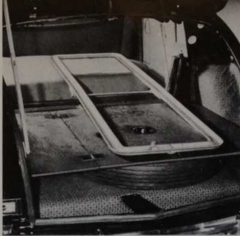
STRETCHER TRACK is shown in place, one end resting on rear seat cushion and other end supported by special plywood shelf over spare tire in trunk compartment. Shelf is secured in place by a single winged nut.
