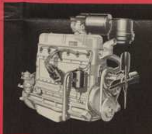
THE POWERFUL VALVE-IN-HEAD Nash "Ambassador" Engine
