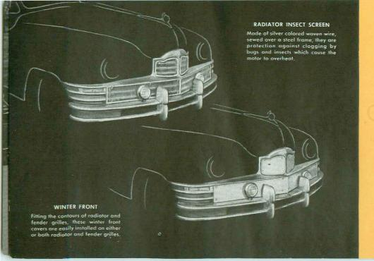
In winter efficient operating temperatures are quickly reached when the cold airstream over the motor is controlled by winterfront covers. Quick warm-up prevents excessive wear of all moving engine parts.
