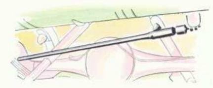
Packard suspension adjusts itself automatically to changes in load and road . . . and there's a fifth shock absorber to damp out side-to-side tremors.
