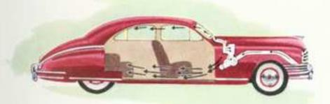
New Comfort-aire ventilation provides a controlled flow of fresh air in any weather.
