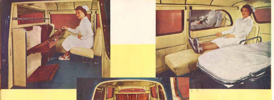
The Cabinet in the Henney-Packard Ambulance has been designed and engineered to provide storage space for needed supplies such as first aid and sanitary equipment.
