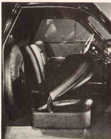
Right cushion back tilted forward to furnish easy access to spare wheel.
