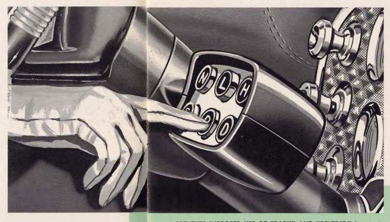
PREVENTS IMPROPER USE OF "PARK" AND "REVERSE." Ingeniously engineered built-in safety system automatically cancels out reverse, park and neutral circuits when car is moving faster than a walking speed. If a child accidently reaches over and pushes a button, nothing happens. And once again, Packard leads the way to freer, easier and safer driving.
