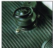
Floor-mounted wiper/washer control. A two-pressure foot-operated wiper/washer, Press lightly and the wipers wipe the screen. Press harder and the windscreen washer sprays it clean. All done with one foot. Hands on the wheel. Safely.
