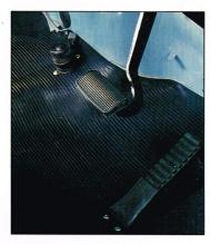
Brakes with pendant pedals. You stop sure and straight in Transit—thanks to direct acting hydraulic brakes all round. Direct acting servo brakes are standard equipment on Custom Buses and optional equipment (at extra cost) on all other models. Pendant type pedals for greater comfort and safety. Front
