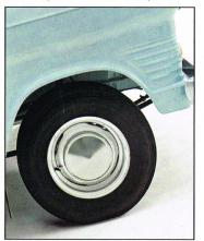
Wheels and tyres. Pressed steel disc wheels come with painted hub caps on short wheelbase models (chromed hub caps on Custom SWB models). Car size (14 in.) tyres make sound business sense. You get high weight-carrying capacity, low loading height and good tyre wear. Wide choice of tyres—including cross-plys and long-life radials—to fit your loads and roads. Choice helps a fleet buyer to standardise tyres on all his vehicles.
