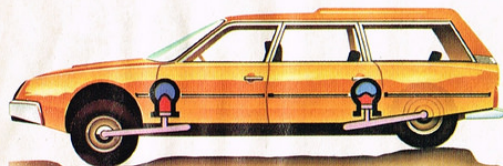
Hydropneumatic suspension maintains constant ride level regardless of road surface and load.
