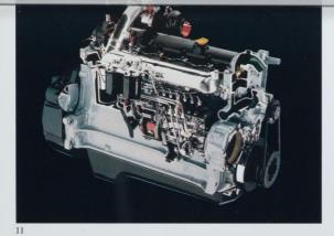
The Garret turbocharger and Bosch high pressure direct fuel injection
