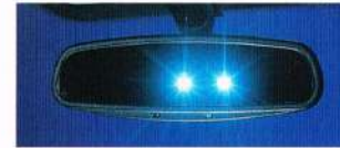
The Ultima's electrochromatic rear view mirror operates by continually sensing light on its surface.
