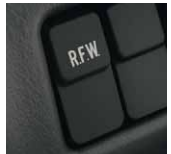
4x4 remote free wheel hubs can be disengaged at the touch of a button.
