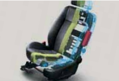
Seat engineering Mondeo's seats have comfort and safety built-in. All seats have anti-submarining bases as standard, while the front seats incorporate side thorax airbags and anti-whiplash head restraints.
