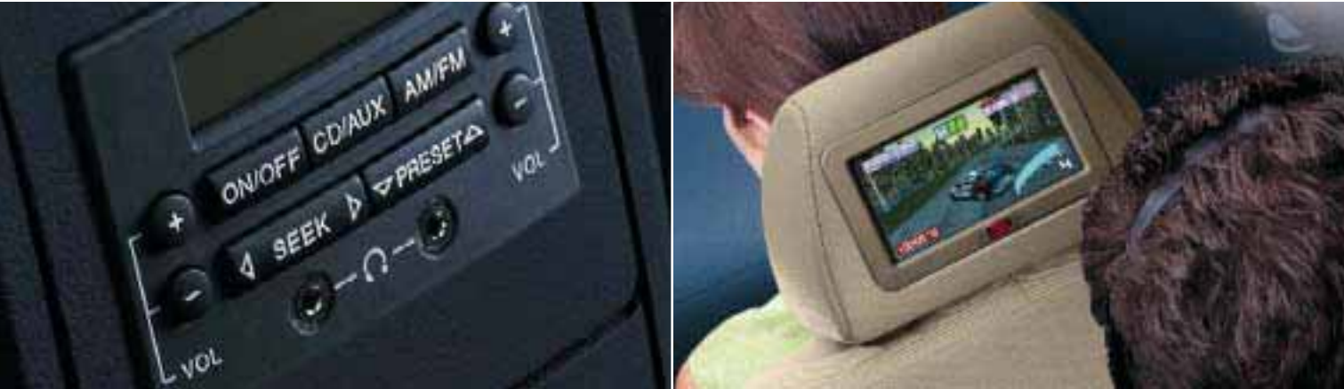
Rear seat audio system Features independent audio controls for the rear seat passengers, plus two headphone sockets. Requires Sony audio system or DVD navigation system with touch-screen.
