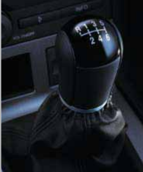
Durashift 6-speed manual transmission The new Durashift 6-speed transmission combines greater in-gear flexibility and top speed potential with enhanced fuel economy and refinement.
