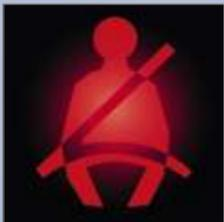
A light and sound indicator gives a warning if the driver seat-belt is not fastened once under way.
