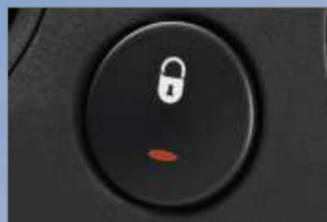
The central locking button instantly locks or unlocks the doors and boot. At speeds greater than 6 mph, the central locking operates automatically.
