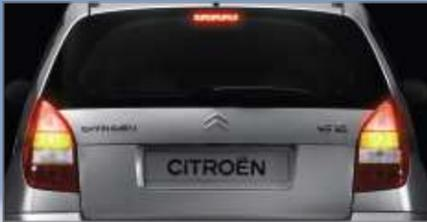
In the event of rapid deceleration, the hazard warning lights are automatically activated to alert other drivers.
