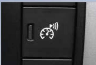
A clever control† located on the central console enables you to register a maximum speed. In the event of exceeding this pre-programmed limit, an audible warning will alert you.
