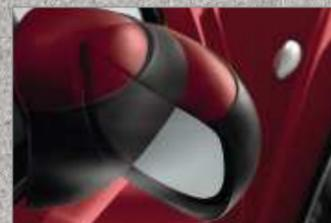
Door mirrors<sup>†</sup> are electrically adjustable, heated and can be automatically folded in tight conditions.
