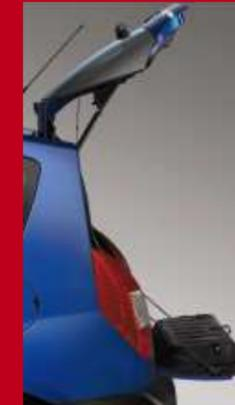
When open, the lower tailgate provides a platform on which to place heavy objects (up to 100 kilos) or to sit down.
