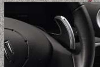
SensoDrive gearbox<sup>†</sup> allows you a choice of driving style – manual or fully automatic. Reacting faster than the most experienced of drivers in just a fraction of a second, manual gear change can be operated either by fixed column mounted paddles located behind the steering wheel or by the floor mounted gear lever with a forward and back movement.
