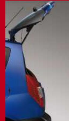
The upper tailgate opens in a single movement to give complete access. And the minimum clearance needed is just 15 cm – very handy when parking conditions are tight.
