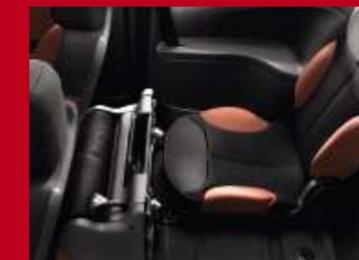
The seat can then also swing up 90°, assisted by gas struts creating a massive 879 litres of storage space when both rear seats are folded.
