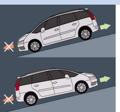
The C4 Picasso's automatic electric parking brake improves comfort and safety. This electric brake is automatically applied when the engine stops. The ECU works in tandem with the ESP to calculate the force required to immobilise the vehicle, depending on the gradient of the road. As soon as the torque applied to the drive wheels is sufficient, the parking brake is automatically released.
