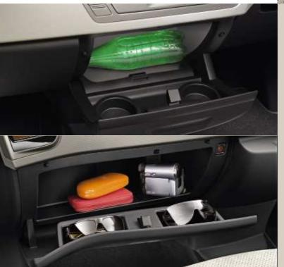
Models with the six-speed Electronic Gearbox System are designed for more space with an extra storage compartment positioned on the lower central part of the dashboard. This compartment is also a cooler and will keep products such as a 1.5 ltr bottle and two 0.5 ltr bottles at a low temperature, even when the air conditioning blows hot air into the cabin. Simply open the compartment and the lid becomes a tray with two cup-holders.
