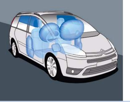
In the event of an impact, the C4 Picasso features a steering column airbag protecting the driver's knees and shins. Thanks to the fixed-centred controls steering wheel, the driver's airbag is designed to be deployed at the required, precise angle for optimal protection. Further protection is built-in so that the pressure and volume of the airbag automatically adjusts with the force of collision.
