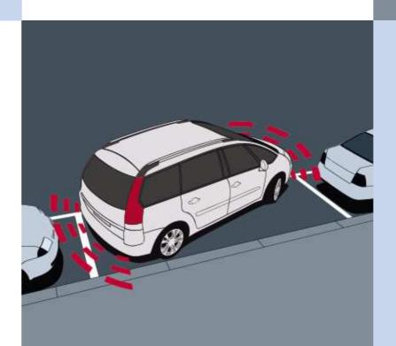
The C4 Picasso features a smart thinking parking space 'gap' measurement system that uses two ultrasonic sensors located at either end of the front bumper. This informs the driver whether the space available is large enough as well as the degree of difficulty of the parking manoeuvre.
