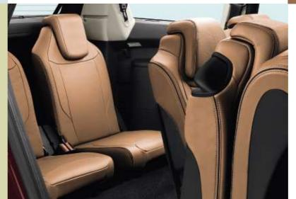
The unique and original moving seat design of the C4 Picasso creates easy access to row three. Activate the control and the cushions to the outer seats in row two automatically lift up towards the seat back. Just slide the seat forward up against the front seat-backs in a single movement and free the space for immediate access to the third row.
