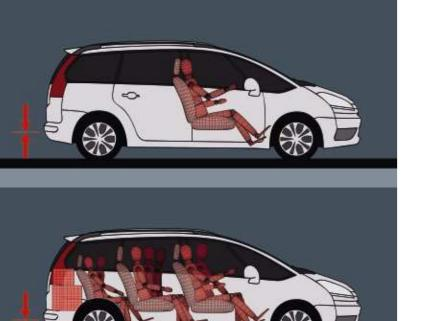
The C4 Picasso can be fitted with a rear pneumatic suspension system that offers improved comfort for all passengers and a constant height no matter the load. The clever pneumatic suspension system at the rear enhances passenger comfort by making suspension smoother and damping the force applied to the C4 Picasso over irregular road surfaces. Heavy load or light load, the C4 Picasso maintains stable vehicle attitude for a more pleasurable and safe drive.
