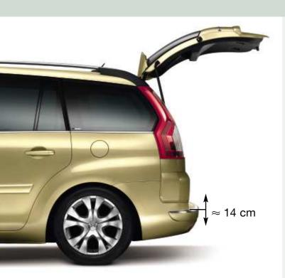
When it comes to state of the art pneumatic suspension, look no further. Press the control button in the boot and lower or raise your stationary C4 Picasso up to 7cm, making it easier to load heavy or large objects. The C4 Picasso can then be easily returned to its original height, either manually by pressing the button twice or automatically, when the vehicle exceeds a speed of 6 mph.
