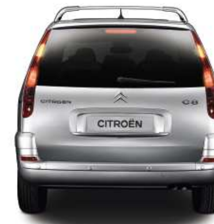
In the event of sudden and strong deceleration the hazard lights are automatically activated, giving the drivers behind a timely warning.
