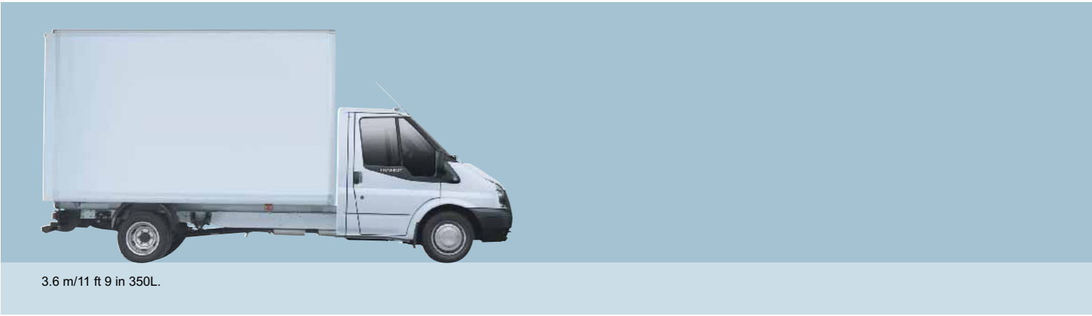
Optional Luton head. One piece GRP Luton head provides useful additional stowage above cab. Bolt on design enables easy repair or replacement.
