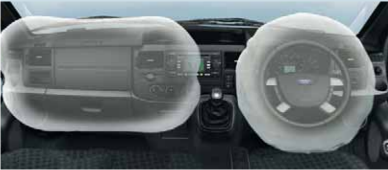
Passenger's airbag * is designed to cushion occupants in a frontal collision. (Option)
