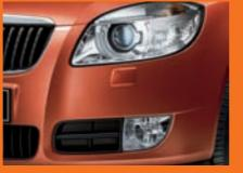
**Cornering front fog lights (optional)** When driving at low speeds and turning the vehicle into a road or at a junction, the 'corner' function illuminates an additional area of the road to the side of the vehicle, increasing visibility for the driver.
