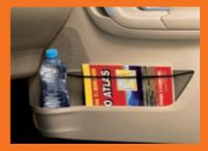
Clever Škoda touches Holders in both front door panels for 1.5 litre bottles and a clever elastic strap for holding items in place are examples of some of the many clever touches on the New Fabia.
