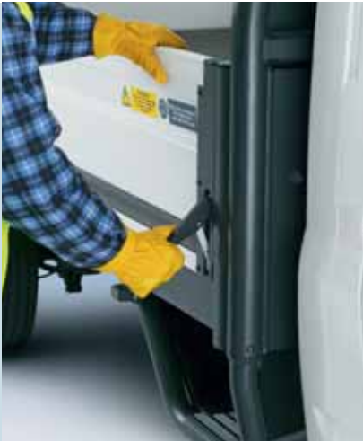
Easy to operate overcentre cam latches provide secure board retention.
