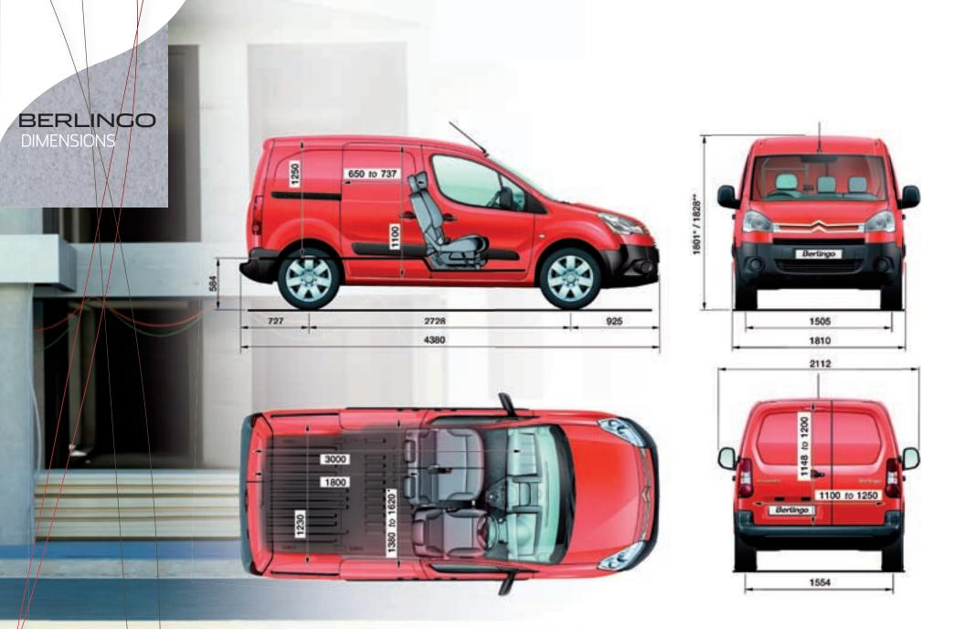
\* 625kg version. \*\*850kg version. \*1620mm without sliding side loading doors, 1500mm with one sliding side loading door and 1380mm with twin sliding side loading doors. All measurements are in millimetres.
