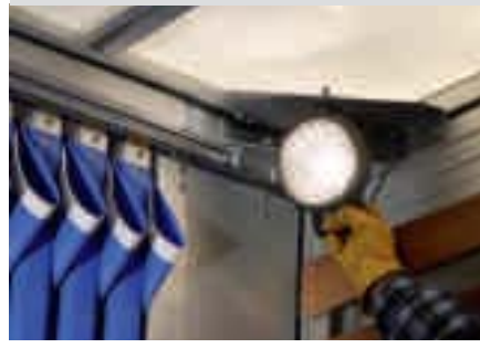
Flush fitting pull-up load anchorage points, 4 per side mounted discreetly into the curtain lower runner section
