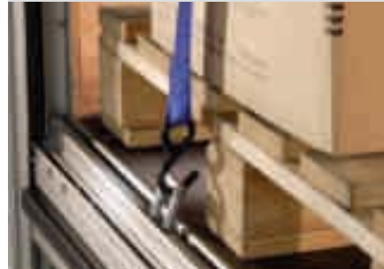
Flush fitting pull-up load anchorage points, 4 per side mounted discreetly into the curtain lower runner section
