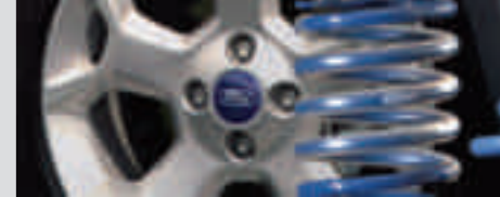
Eibach suspension-lowering kit Enhances driving performance and handling as well as giving a more sporty appearance. Lowers the car by approximately 30 mm. (Accessory)
