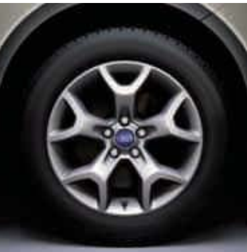
Alloy wheel – 17", 5x2-spoke, 235/55 tyres. (Standard on Zetec)
