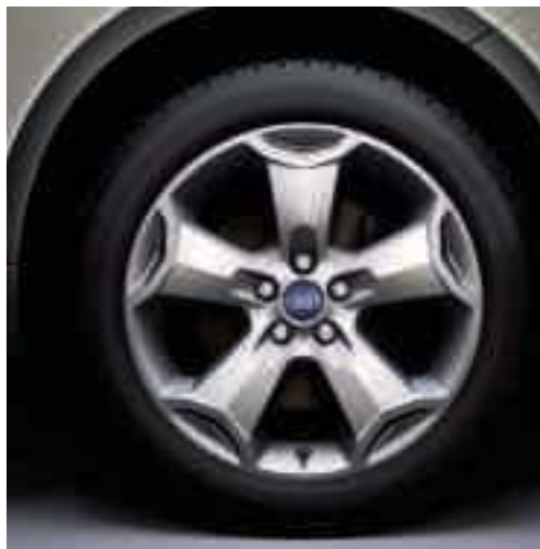
Alloy wheel – 7.5x18", 5-spoke, 235/50 tyres. (Option and dealer fit accessory)
