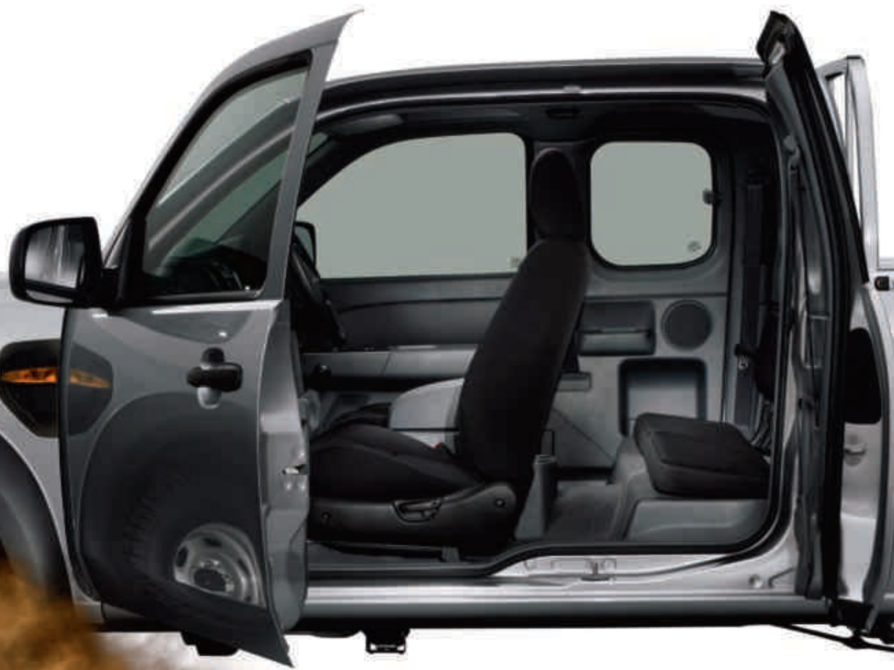
Super Cab Four door cab style with reverse-hinged rear doors and seats for up to four occupants.
