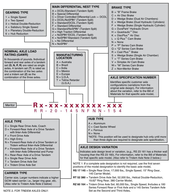
NOTE 3: The term "Tandem Split" refers to when there is a difference between the Forward axle and Rear axle of the Tandem or Tridem axle set when the Tandem or Tridem axle set part number is used. The value to the left of the "/" references the Forward axle, and the number to the right of the "/" references the Rear axle. For information related to the Middle axle of a Tridem axle set part number, refer to the Bills of Material.
