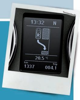
• The driver is responsible for the manoeuvre at all times. The manoeuvre is cancelled if the steering wheel is touched or the speed exceeds 4 mph.
