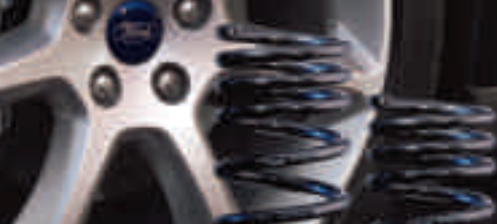
Eibach suspension-lowering kit Enhances driving performance and handling as well as giving a more sporty appearance. Lowers the car by approximately 30 mm. (Accessory)
