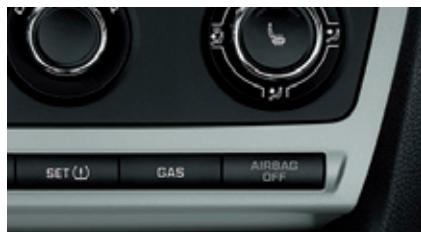
The vehicle is installed with both automatic and **manual switch** to shift between the two fuel modes. The manual switch is performed by the **GAS button** and may be used while the engine is running, even when the car is moving.
