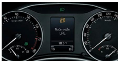
When the vehicle is fueled by LPG, the **light on the instrument panel** is active. The amount of LPG remaining in the tank is clearly indicated by a **fuel level needle**. If the LPG supply is reduced to the reserve level, the **informational display** notifies you in time of the need to refuel.
