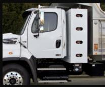
CNG tanks mounted back-of-cab.
