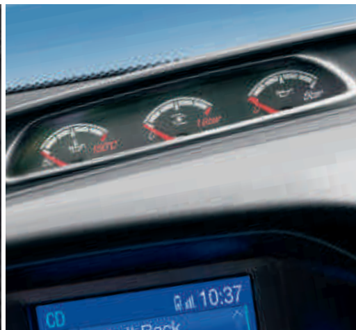
Unique ST instrument cluster binnacle Featuring turbo boost, oil pressure and oil temperature gauges. (Standard)
