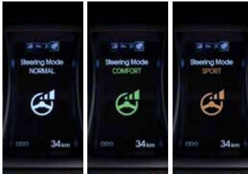
With optional Flex Steer you can adjust the steering performance to your personal driving style: it includes Comfort mode for easy parking and urban driving, Normal mode, and Sports mode for motorway driving.
