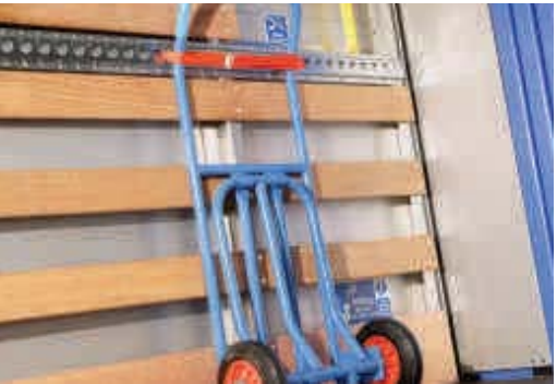
Load-loc rail Optional bulkhead load-loc rail and additional laths, 6 fitted as standard.
