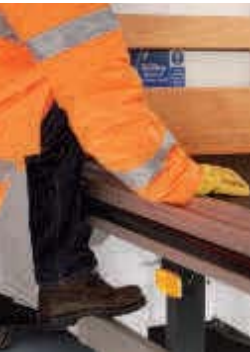
Grab handle and step Standard nearside bulkhead mounted grab handle with optional side underrun guard step, tubular stirrup step fitted as standard.
