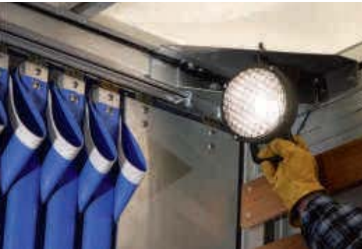
Interior worklamp Halogen worklamp mounted on a ball and socket joint can be repositioned to suit lighting requirements.
