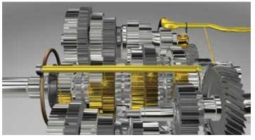
Precision lube system eliminates oil cooler and reduces remaining transmission inefficiencies by nearly one-third.
