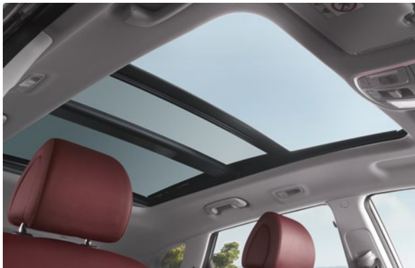
Sunroof – panoramic glass electric tilt & slide (Premium SE). The extra-large sunroof adds the feel of open-air driving. At the touch of a button you can fill the interior with fresh air and sunlight. An automatic wind deflector minimises noise.
