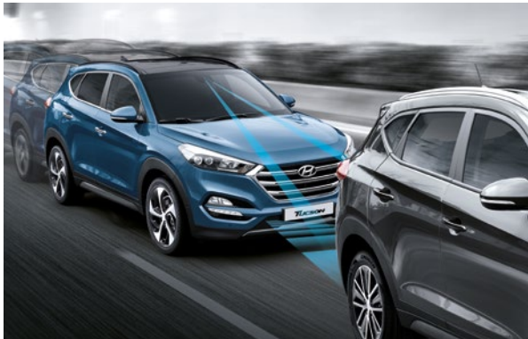
Autonomous Emergency Braking (AEB) (Premium and Premium SE). The radar and camera based Front Collision Warning System (FCWS) alerts the driver of potentially dangerous proximity of vehicles and pedestrians and brakes autonomously if required.
