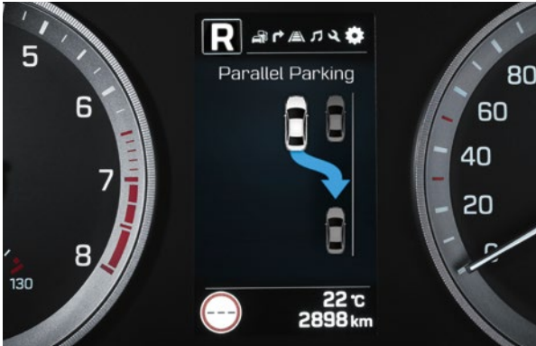
Parking System – Smart Park Assist (Premium SE auto). Activated sensors can identify a viable parallel parking space, and steer the Tucson perfectly into the space. SPAS also steers the car into right angle spaces. You control the pedals, the system does the rest.
