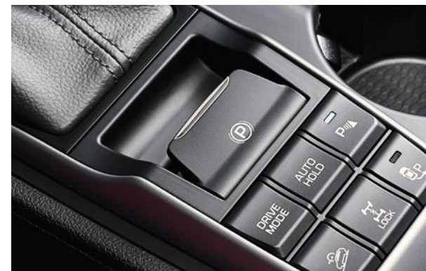
Electric parking brake (Premium auto and Premium SE auto). The compact parking brake control frees up useful interior space between the front seats.
