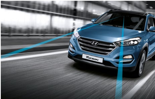
Lane Departure Warning System with Lane Keep Assist (SE, SE Nav, Premium and Premium SE). Instant visual and acoustic warning, plus corrective steering intervention, when unintentional lane departure is detected.
