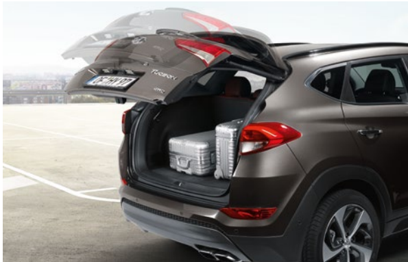
Smart Electric Tailgate (Premium SE). Sensors detect the approach and presence of the key-carrying driver and the tailgate automatically lifts open to provide effortless access to the generous load space.
