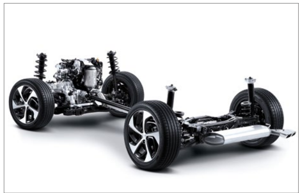
On-demand 4WD (selected models). When a potential loss of traction is detected, up to 50% of torque is transferred to the rear wheels for improved grip on loose, slippery surfaces and enhanced cornering performance. Torque distribution can be locked in 50:50 mode in extreme conditions.
