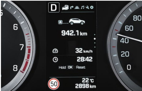
Speed Limit Information Function (SLIF) (SE Nav, Premium and Premium SE). The system recognises roadside signs, cross-checks with navigation data and displays the current speed limit in the navigation screen and the high-resolution TFT display.
