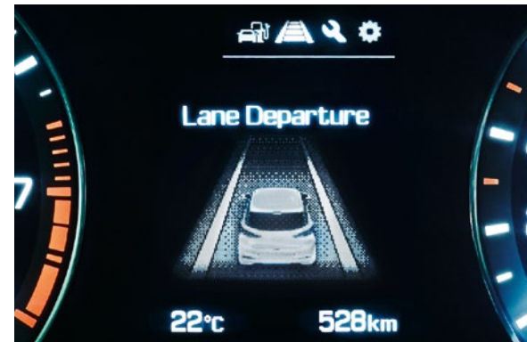
Lane departure warning system. Instant visual and audible warning of unintentional departure from the lane you're driving in. (SE, Premium & Premium SE)
