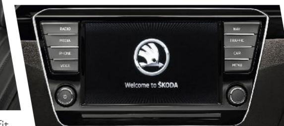
The Columbus navigation system offers comfortable touch control on an 8" colour TFT display. It has two SD card slots, a DVD drive and includes integrated Wi-Fi as well as SmartLink†.
