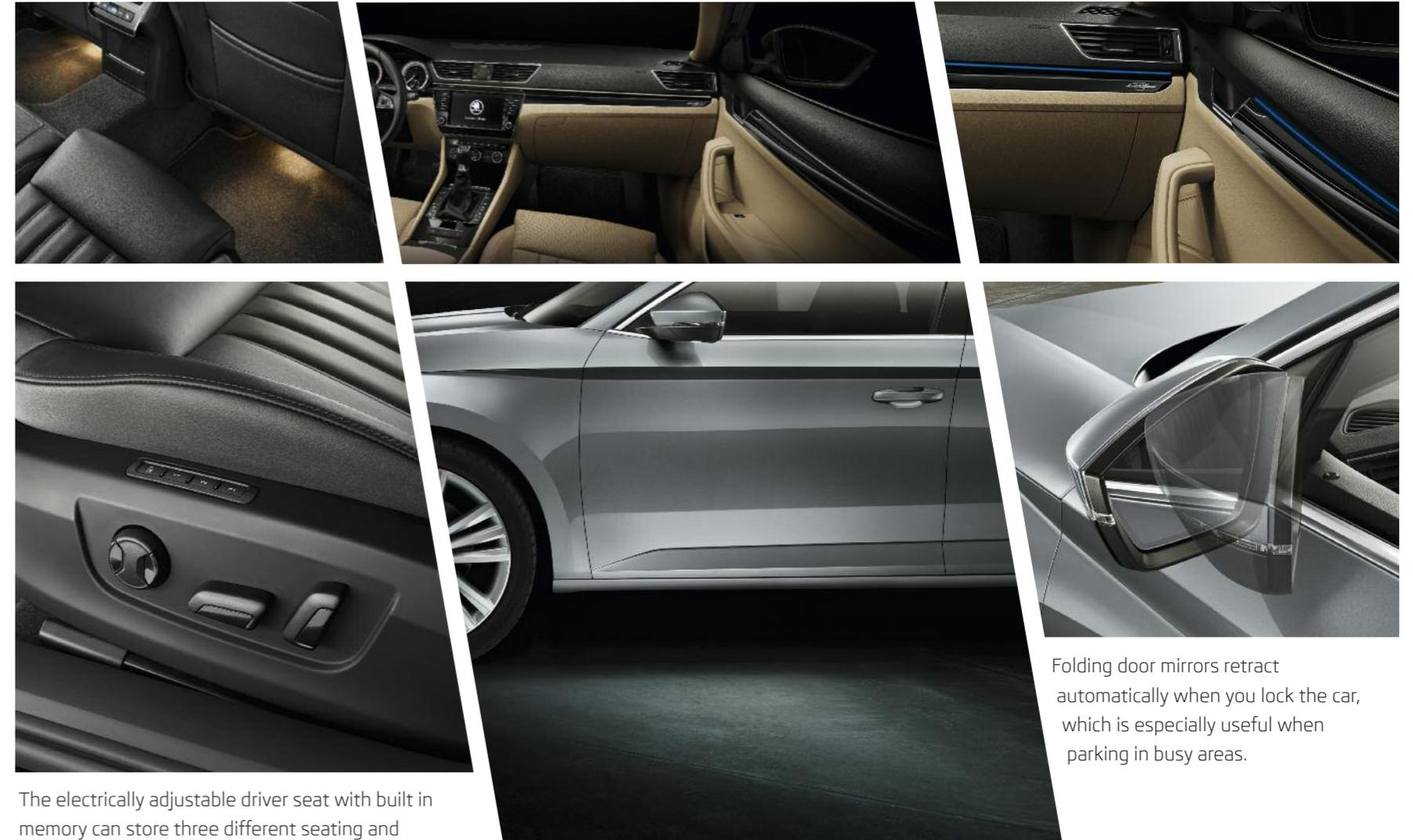
The electrically adjustable driver seat with built in memory can store three different seating and door mirror positions.
