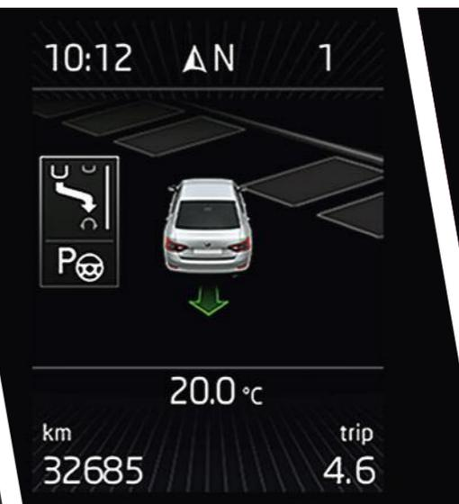
Minimise the hassle of parking in tight spaces with Park assist. It automatically selects an appropriate parking place in a row of parallel or perpendicularly parked vehicles. When parallel parking, it only needs a space 60 cm longer than the car itself.
