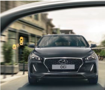
Blind-Spot Detection (BSD) warns of the presence of vehicles hidden in blind spots by means of visual and acoustic alerts.
