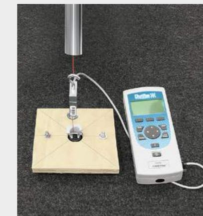
Testing of fixing element strength
