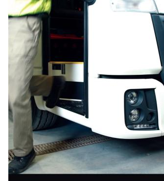
The unique low-entry concept includes a kneeling and lifting function which further reduces an already low step-in height by another three inches.
