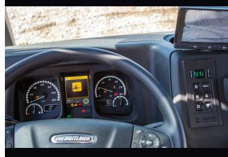
Steering wheel controls allow drivers to cycle through key information displayed on an intuitive LCD screen on the dash.
