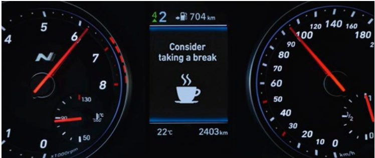
Driver Attention Warning (DAW) . This standard feature raises safety and convenience to an entirely new level by continuously monitoring and analysing driving patterns. When a pattern of fatigue or distraction is identified, DAW gets the driver's attention with an audible alert and pop-up message suggesting a break.
