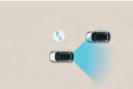
Blind Spot Collision Warning (BCW): Radars detect traffic in the vehicle blind spot, warning drivers with an audible alarm when the indicator is used so you can be aware of the traffic around you even when you can't see it. Standard on Ultimate trim only.
