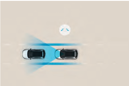
Lane Follow Assist (LFA): Smart sensors and the forward-facing camera detect when the car drifts from the centre of the lane, applying steering torque to maintain road positioning for safety. The car also estimates the trajectory of the vehicle ahead and adjusts its position accordingly. Standard on Ultimate trim only.
