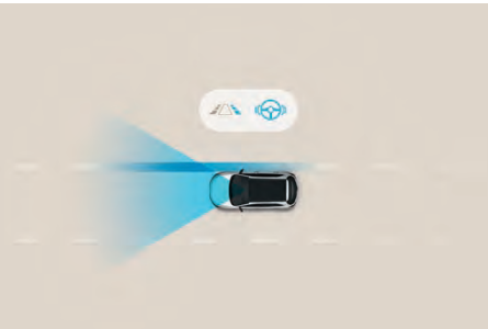
Lane Keeping Assist (LKA): Front multi-function camera is used to monitor the lines of the road. In case of an unintended lane departure, it warns you and can apply counter steering torque to guide the car back to the lane.
