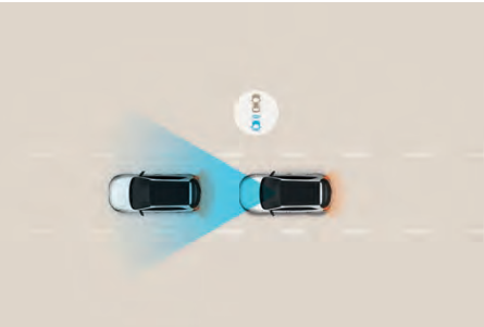
Front Collision Avoidance (FCA): The front view camera and radar sensors warn drivers of imminent collisions with cars, pedestrians and cyclists, applying the brakes when necessary to avoid collisions.
