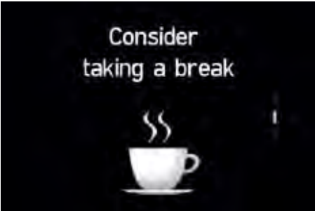
Driver Attention Warning (DAW): When a pattern of fatigue or distraction is identified, the system gets your attention with an alert and pop-up message suggesting a break.
