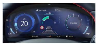
Fiesta EcoBoost Hybrid displays how much electrical power has been generated by the mild-hybrid system, and tracks whether energy is currently being returned to the battery or used to assist fuel efficiency or performance.
