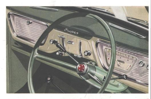
The padded facia places instruments directly in front of the driver. The "stalk" to the right of the steering column controls the direction indicator and the horn, and the one to the left, the dipper. A short floor-mounted lever operates the new 4-speed, all-synchromesh gearbox. The soft, carefully shaped front seats are entirely new, and the revised trim includes rear quarter armrests.
