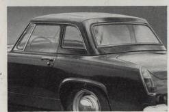
The hood of the Sprite Mk. IV is made of tough, vinyl-coated fabric and fits snugly round the cockpit so that the wind-down windows and hinged louvres can be used to provide the same ventilation and rain-proof comfort of a saloon car.
